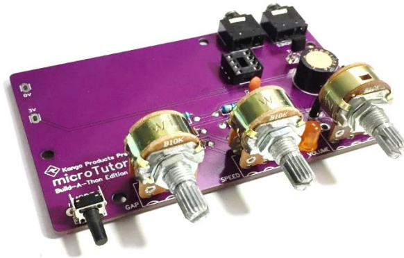
Volume/ Power Switch All Controls Fitted
