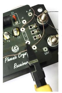
The two white wires need to be trimmed and soldered to the position marked 'L1' on the board, these wires have a very thing insulation on them that will burn off when you solder them in place.
