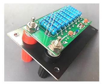
Now place the LED though the PCB board but do NOT solder it yet. Note the LED is fitted on the other side of the board than the resistors. Make sure the LED is fitted the correct way. The long lead goes into the round hole (Marked +). Carefully lower the front panel into the PCB, the ends of the terminal posts should pass through the board. Use the remaining nuts to secure the PCB to the posts. Now push the led up and through the front plate. Solder the led in place.
