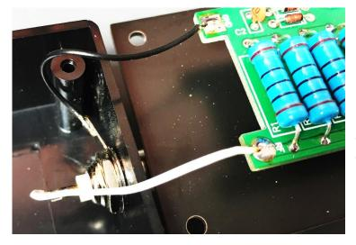
Place a test meter across the BNC input on the left hand edge of the board, the RF input. You should measure 50 ohm (plus or minus 1 ohm).
