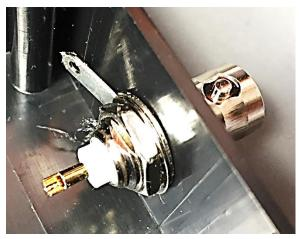
Now fit the BNC socket to the case, You may find it better if you can solder two 50mm wires to the socket (one to the centre pin, one to the tag) before you assembly it onto the case. Take care with this stage and don't hurt your fingers when tightening the BNC. Ideally use a BNC wrench to hold the BNC and stop it from turning while you tighten the rear nut, don't forget to fit the earth tag.
