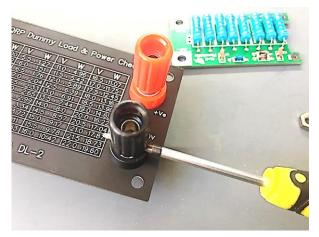
that the posts are installed truly vertical or the PCB will not fit.
