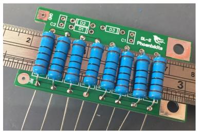
First fit the 8 power resistors (R1 to R8). When fitting these try to leave a small gap between the bottom of the resistor and the Circuit Board. This will help to keep the resistors cool. I insert a thin metal ruler under them before I solder in place so that I can keep a constant gap on all of them.
