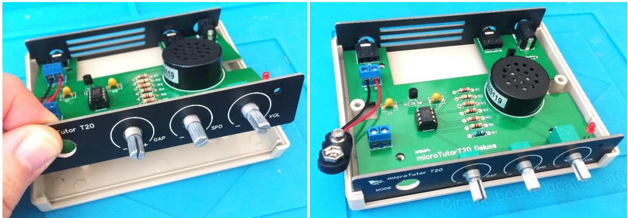
You have two lengths of foam tape, Take the white one and peel the backing from the one side, the side to peel is the plastic finish side , not the paper. Fit this on the bottom case in the cutout area (this is to stop the battery from moving around.)
