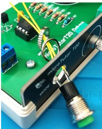
Now fit the switch, this is a little fiddly so take your time. And when fitted cut the loop and wire the two end to the terminal block just behind the switch.
