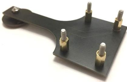
Now find the 4 brass standoffs and the 4 long M3 screws you have left. Put the screws through the key panel top plate and tight the standoffs onto the screws as per the picture here.
