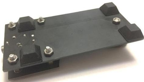
Fit the 4 rubber feet, the front two should be right at the front of the base to help its stability. Put the rear two between the screws on each side.
