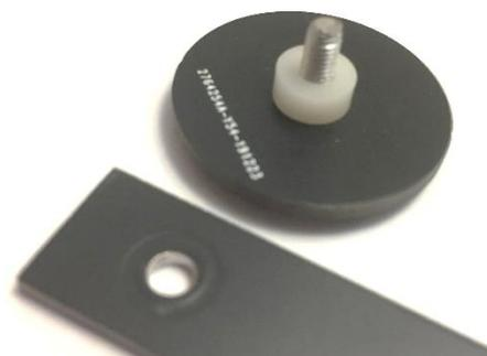
Look at the main key top board and you will note 4 holes at one end and 1 hole on the thinner arm. On the arm the hole has a sliver contact ring on one side of the board This side **MUST** be the bottom of the top panel, the flange mounts so that the nut makes contact with this contact ring. This will form part of the circuit for the key. The screw will protrude by just about 1mm from the bottom of the nut.
