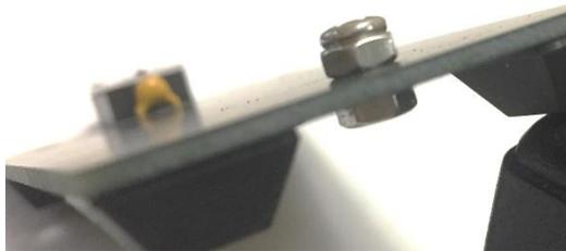
Now fit the bottom contact screw. Find the 6mm Screw (The shortest in the kit) and BEFORE putting it on the bottom board put one of the M3 nuts onto the screw, tighten this nut onto the screw. Put the screw through the single hole at the one end of
