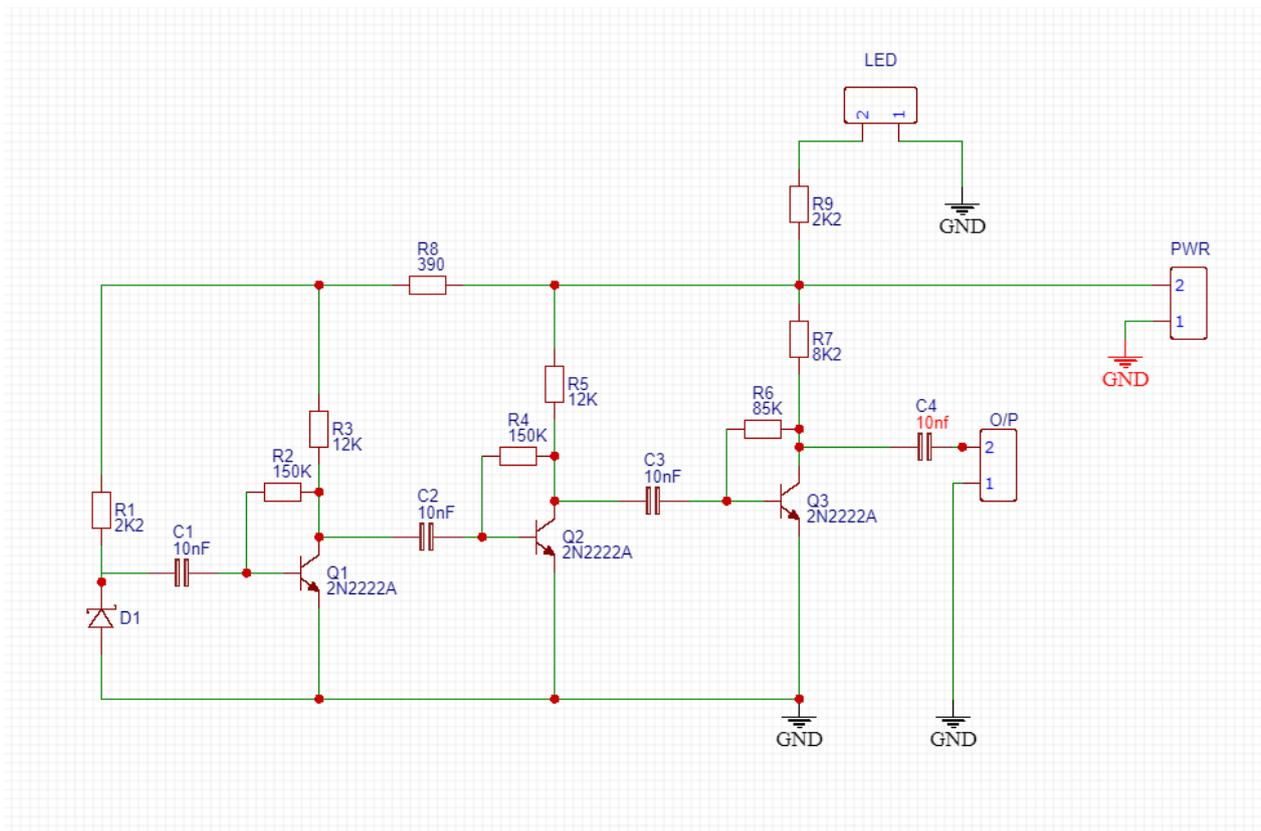
Here you can see the noise source is a small Zener diode, the exact value isn't critical anything from about 5 to 7 volts will do the trick. The noise from the diode is past via C1 to the first transistor, this and the following transistor act as amplifiers and the amplified signal is available just after C4.
