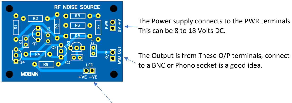
The 'Power On' Indicator led can be wired to here if you wish to use one. The resistor for it is already fitted (the Long lead on the LED is connected to +VE).
