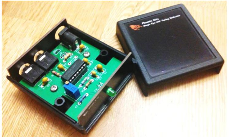
The user can set the frequency that the Magic Eye will respond to from around 450Hz to 1Khz so just about all sidetone frequencies can be selected.
